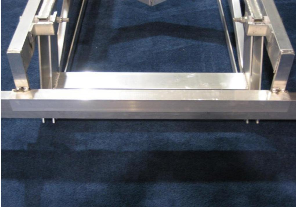
Measure the beams and center the beams on the cradle as best as possible. Using the  $3/8''$  x  $6 - 1/4''$  x  $3 - 3/4''$  U-Bolts attach the front and rear beams by using the  $3/8''$  flange nuts as shown in the picture below:
